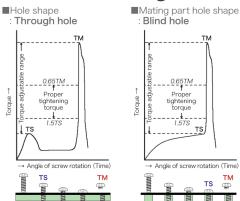
TS...Thread forming torque TM...Failure torque
