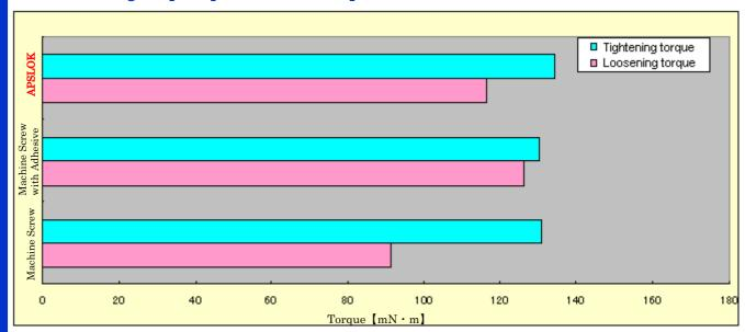
Note: Machine screw with adhesive is measured loosening torque at 24 hours after fastening.
