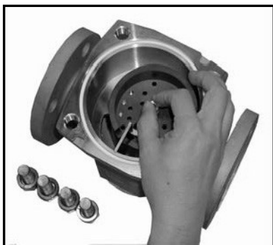
Check if the rotor turns smoothly. If it is hooked, biting of foreign matter is suspected. Remove the foreign matter.
