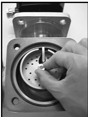
Check if the rotor turns smoothly. If it is hooked, biting of foreign matter is suspected. Remove the foreign matter.
