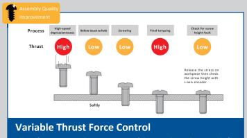
Allows for accurate and precise setting of thrust and travelling speed of screw-driving tool. Optimum thrust control effectively prevents damage to internal threads and cam-out.
