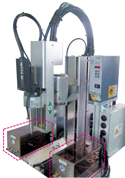
● Screw Driving Robot equipped with 2 DF200 units
