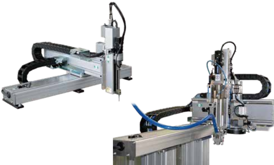
Case of XY (cartesian) robot
