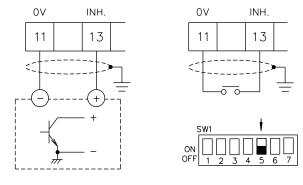
■ Connection of subtraction pulse input
