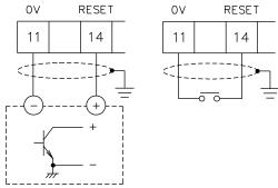
●Connection of inhibit signal (Negative input)
